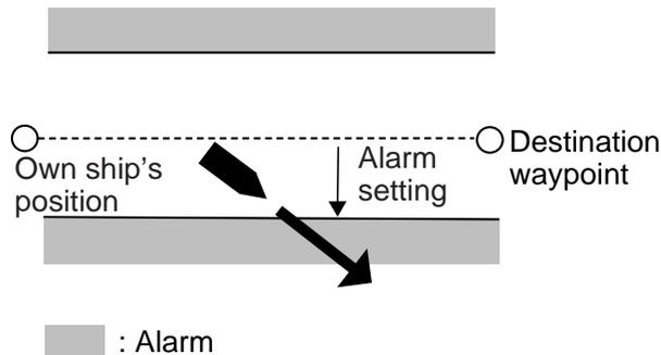
*Figure 6-6 How the XTE alarm works*
