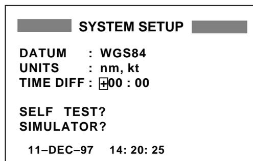
Figure 1-13 SYSTEM SETUP menu, TIME DIFF line selected
