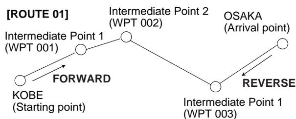
Figure 5-8 Meaning of forward and reverse
