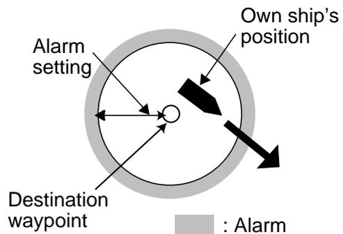
Figure 6-5 How the anchor watch alarm works
