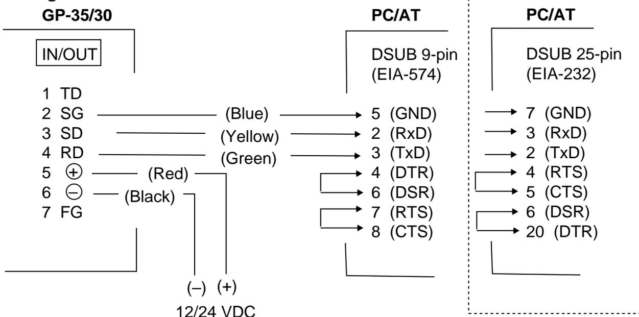
Figure 7-13 Connection of GP-35 to PC
